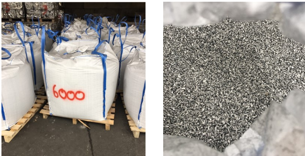
Figure 1. Aluminium granules from end-of-life electrical cables.
